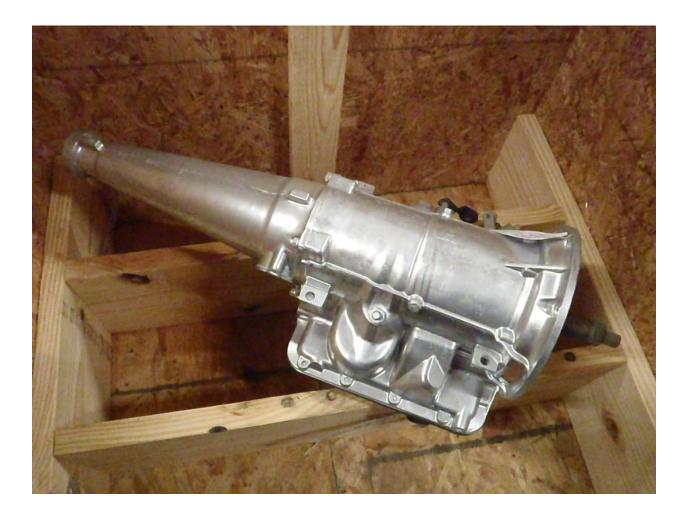
Short shaft cast iron case transmission last used on the car line in the 1957 Hawk.
