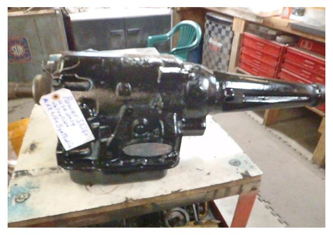
Borg warner model 35 aluminum case transmission used with Studebaker 6cylinder engines 1963 and 1964. A very durable smooth transmission with first gear start
