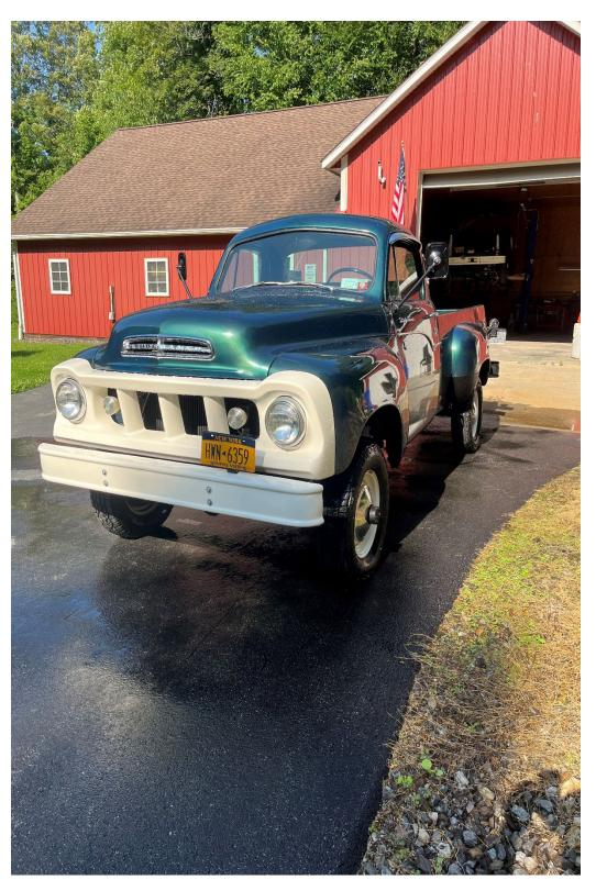
This was one of my favroites.1959 NAPCO 4WD factory equipped with a cloverleaf 289. During restoration the only changes I made was to add a 4 barrel carburetor a large rear bumper and 3:31 gears in the differentials. It made a nice road truck.
